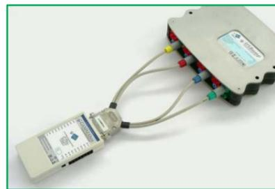
*g-USBamp* works with any type of passive electrodes and strip or grid ECoG electrodes. The *g.GAMMASys* active electrode system can be used as well. Single cell recordings can be performed in combination with *g.tec*'s spike sensor system.
